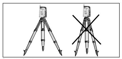
Figure 4.24 Correct instrument set up
