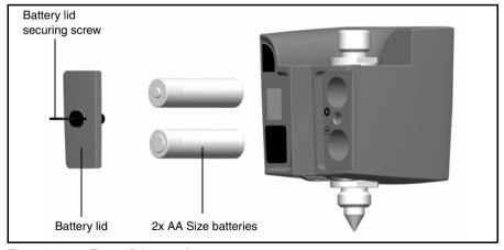
Figure 7.60 Target ID battery change
