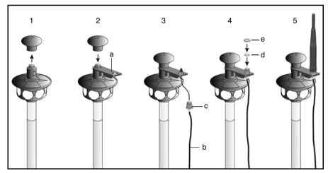
Figure 7.77 Fitting the antenna extension kit.
