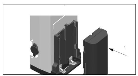
Figure 7.73 Fitting battery to external radio
