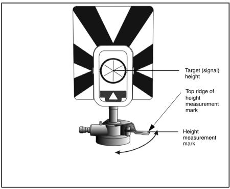
Figure 7.63 Target height marks
