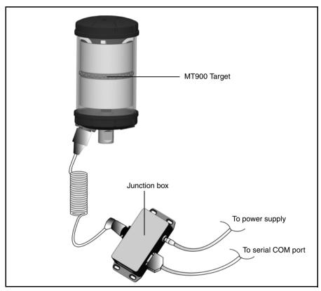
Figure 7.62 Connecting the Junction Box
