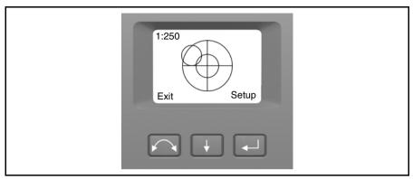
Figure 3.17 Electronic leveling screen on the face 2 display
