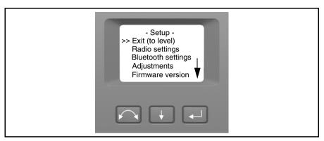
The instrument Setup menu is structured as follows:
