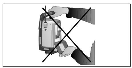
Figure 4.42 Wrong way to lift the instrument
