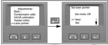
2. To change the laser pointer setting press to select Next and then press to select On or Off
