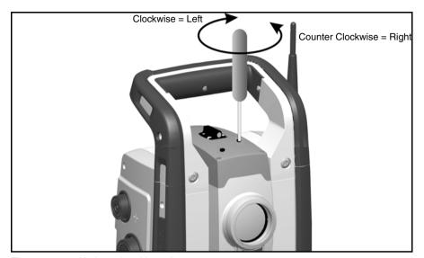
Figure 4.30 Horizontal position adjustment
