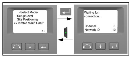
After the selection the instrument will go to suspend mode, to return to the Select Mode menu press the trigger/on/off key.
