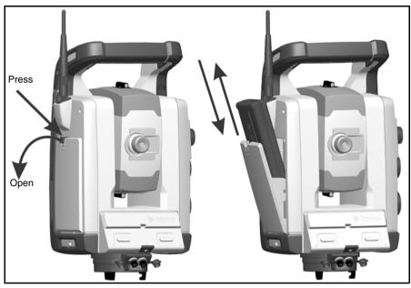
Figure 3.11 Removing and replacing the internal battery
