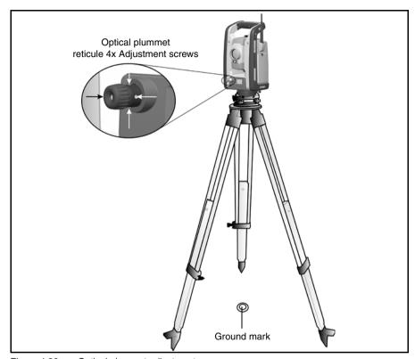
Figure 4.33 Optical plummet adjustment
