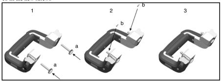
Figure 7.79 Fitting the new screws
