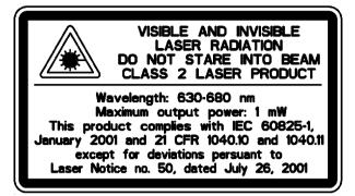
The instrument contains visible and invisible laser sources
