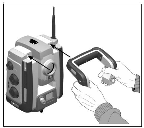
Figure 7.80 Attaching the handle
