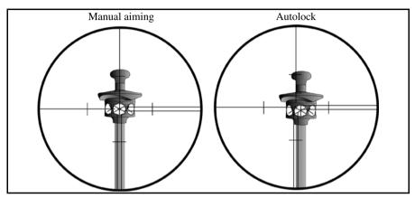
Figure 7.55 Difference between aiming manually and Autolock
