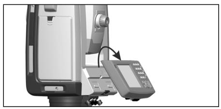
Figure 4.37 Detaching the Trimble CU
