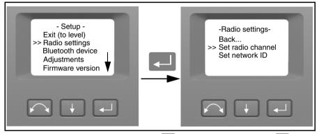
**3.** To change the radio channel number press to select Next and then press change the channel number in the display.
