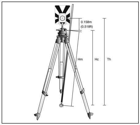
Figure 7.64 Target height measurement
