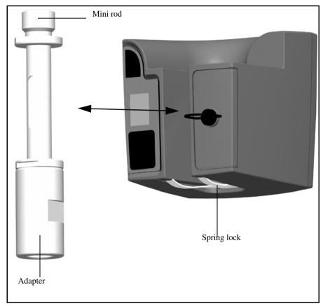
Figure 7.58 Fitting or removing the Target ID.
