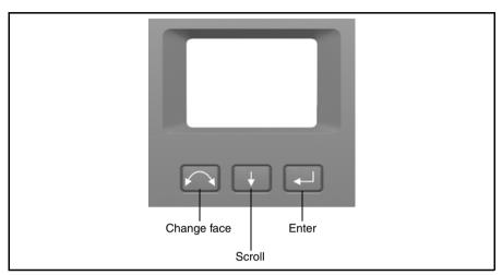
Figure 3.16 Face 2 display and keyboard
