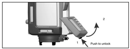
Figure 4.36 Detaching the Trimble CU
