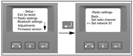
**3.** To change the network ID number press to select Next and then press to change the channel number in the display.
