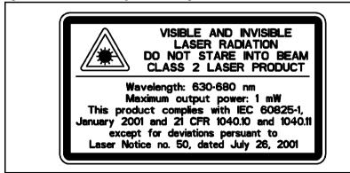
Figure 3.23 Laser pointer warning label
