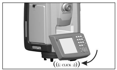
Figure 4.35 Attaching the Trimble CU
