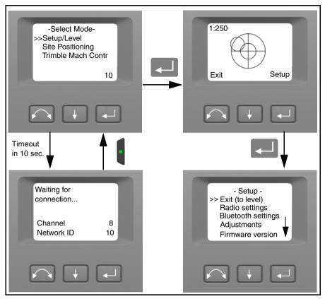
From this menu you can set up the remote operating modes Site Positioning or Trimble Machine Control.
