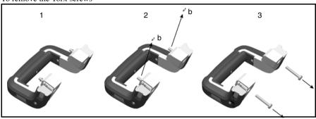
Figure 7.78 Removing the Torx screws
