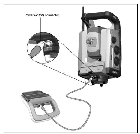
Figure 3.13 Connecting the Multi battery Adapter
