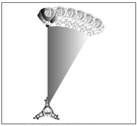
Figure 7.54 The Trimble SPS Series Total Station Autolock function.
