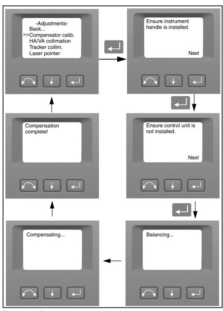
Figure 4.26 Compensator calibration routine
