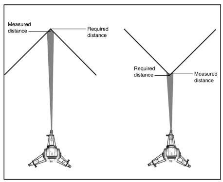
Figure 6.45 Measuring to an inner and an outer corner
