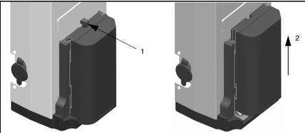
Figure 7.75 Removing battery from external radio
