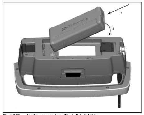
Figure 7.66 Attaching a battery to the Trimble Robotic Holder
