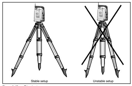
Figure 6.47 Tripod setup
