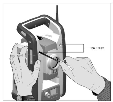
Figure 3.19 Removing the instrument handle
