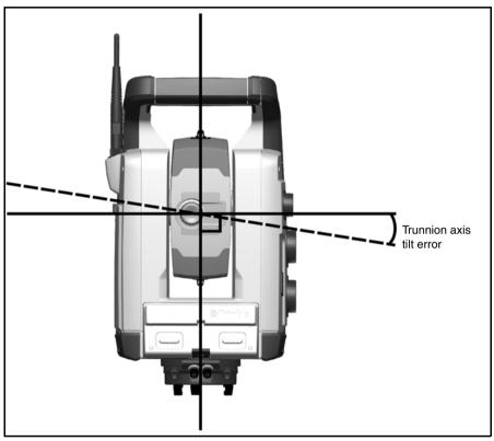
Figure 6.43 Trunnion axis tilt error
