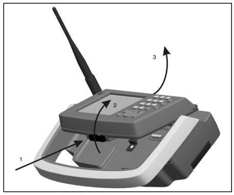
Detach Trimble CU from Trimble Robotic Holder Figure 7.69
