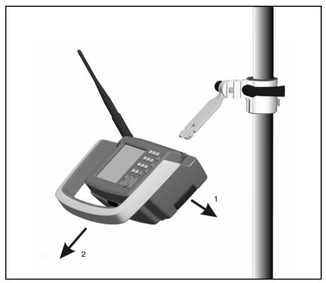
Figure 7.71 Detach Trimble Robotic Holder from stake writer rod adapter
