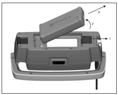
Figure 7.67 Detaching a battery from the Trimble Robotic Holder
