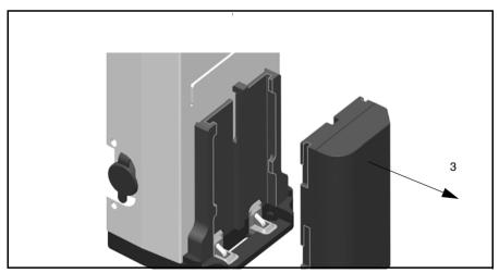
Figure 7.76 Removing battery from external radio
