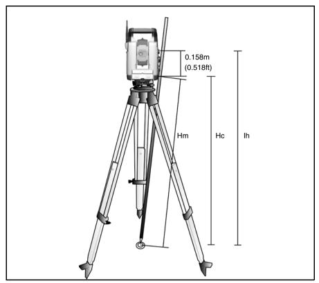
Figure 4.32 Instrument height measurement
